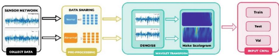
Fig. 4. The block diagram of the proposed damage detection method.
