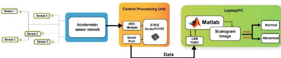
**Fig. 1.** A data collection system diagram for OJP.
