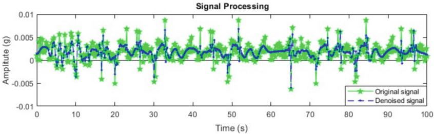
**Fig. 3.** Original signals and denoised signals by wavelet transform.
