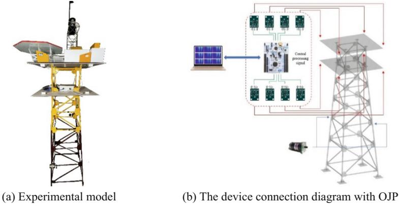
**Fig. 2.** The setup and arrangement of the experimental model.
